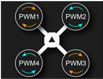
**Motor Wires:** To change the rotation direction you can use the [JP1] solder jumpers on top of the board to match Mot1/CW, Mot2/CCW, Mot3/CW and Mot4/CCW.
